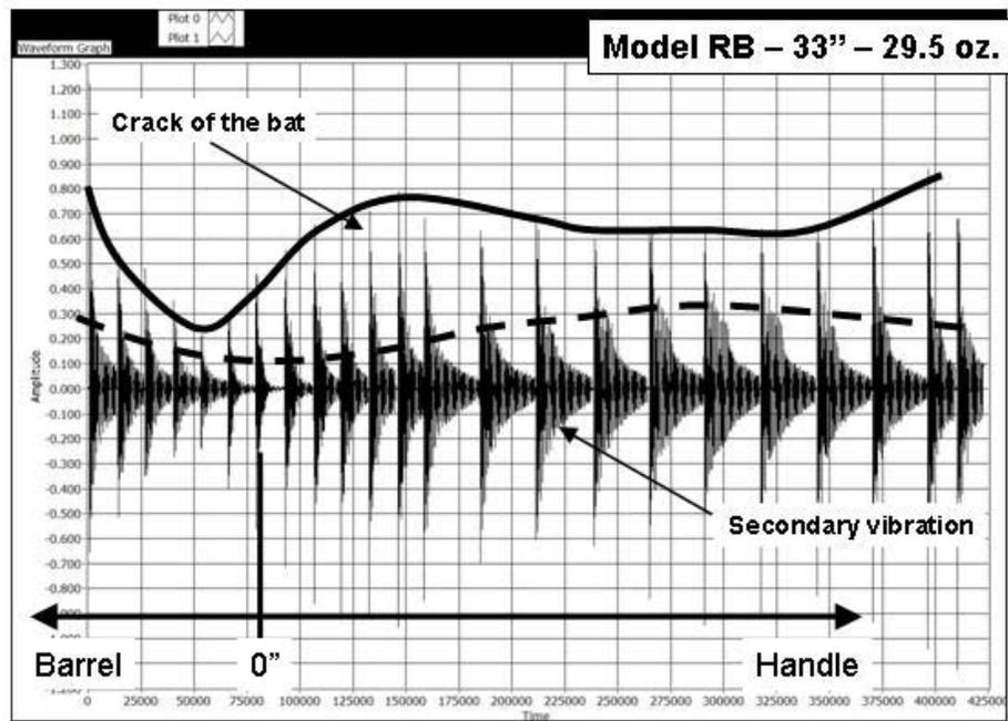
**Figure 2.** Vibration test results for 29.5 oz. RockBat (Lightweight bat).
