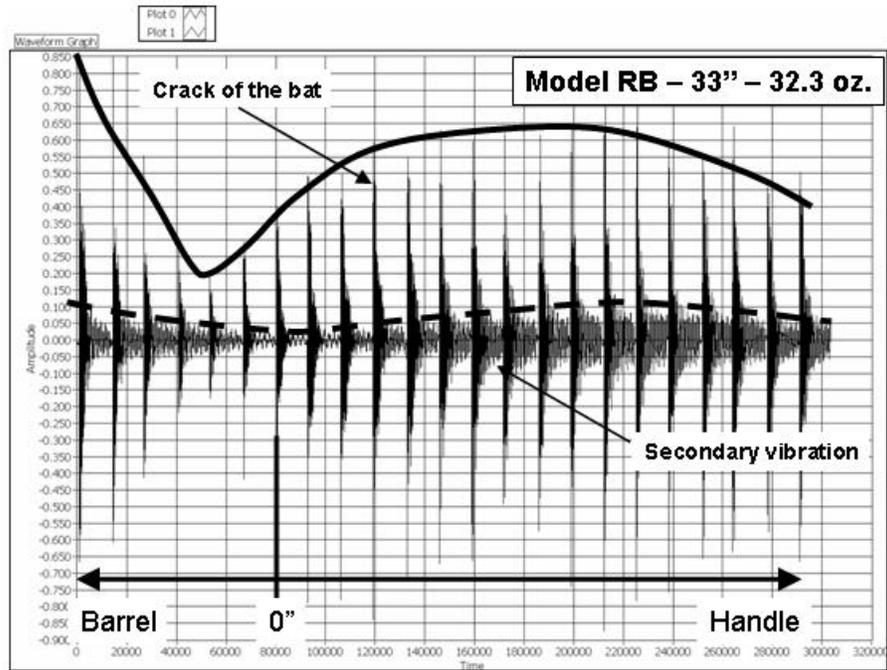
**Figure 1.** Vibration test results for 32.3 oz. RockBat (Heavy bat).
