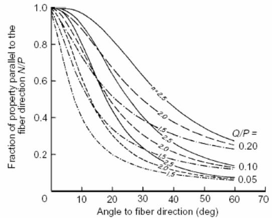
In the above table, the property most related to baseball bat performance is toughness. Furthermore, the Wood Handbook specifically states that impact bending properties fall close to the curve having  $Q/P = 0.05$  and  $n=1.5$ . In the graph above, the curve that best represents  $Q/P=0.05$  and  $n=1.5$  is the absolute bottom curve having the steepest slope.
